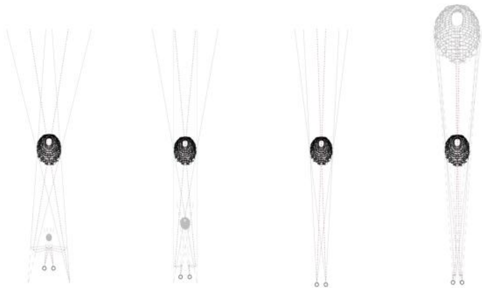
Figure 3: By diverting the visual path using mirrors in the fashion of the tele-stereoscope, the angle under which an item is seen, can be adjusted. As a consequence, the perceived distance and size of the object is altered. A larger angle will show the item smaller and closer, while a smaller angle will make the item appear larger and further away. Drawing by the author.
