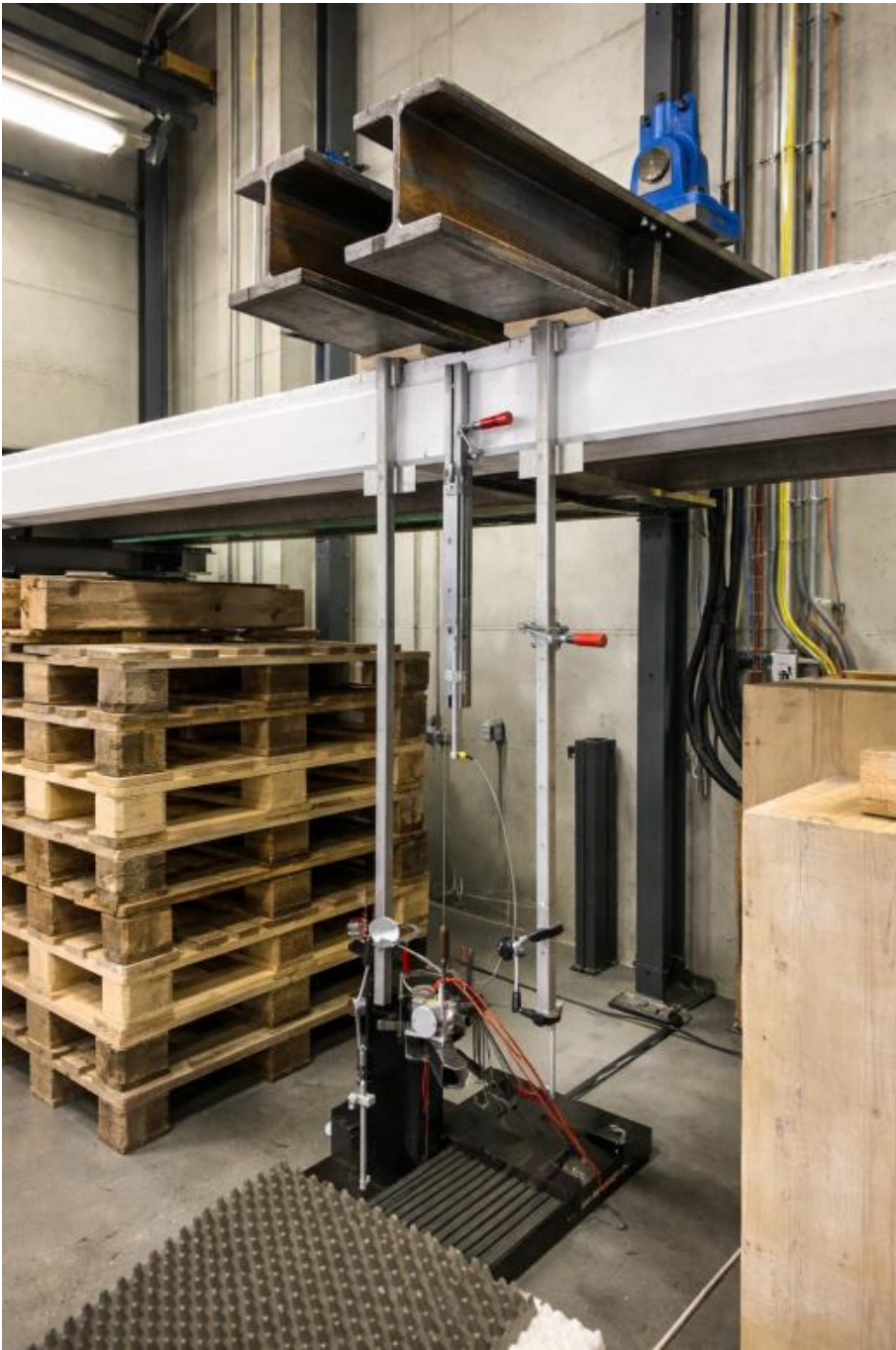
Figure 6: Verification phase of the structural performance of ribbed concrete slabs reused from the dismantling of the Lysbüchel parking garage. Graphic by Parabase. © Parabase, with permission for publication.
